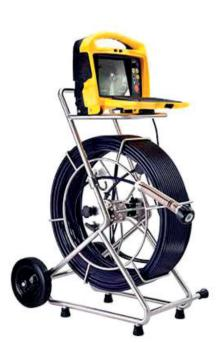
The Vivax vCamMX-2 all-in-one mini inspection system. With either 17mm or 26mm cameras on 30 to 45meter pushrod. The system has multi-frequency sondes, video recording, and 8" screen and a 7-hour battery.
