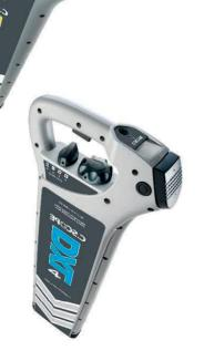
The latest underground locators or cable avoidance tools are truly amazing developments. They have dual frequency working at 33 and 131kHz for maximum exposure of underground plant. The cable avoidance tools have Power, Radio and Generator modes for identify varying types of plant underfoot. The systems use the latest technology to be energy efficient and even have swing alerts to ensure that the systems are used correctly.
