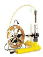
Using a modified C-Scope Flexible Tracer, the Stargland System can be used in Polyethylene mains from 63mm and above through a High Flo 63mm Top Tee for tracing mains up to 160meters from one excavation.
