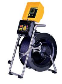
The Vivax vCam6-HD is a full survey system. With either 34mm or 46mm diameter self-levelling cameras on 60 to 120meter pushrods. The system has multi-frequency sondes video recording, and a 9.7" screen and a 4-hour battery.
