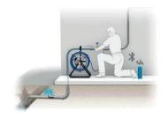
A leak can be identified through the change in noise at the point of the leak. The change in the noise can be listened to through headphones or linked to a high-quality waterproof and shockproof Bluetooth speaker. There is also a visual display via a light bar.
