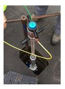
The SynthoCam H<sub>2</sub>O Mic system is made with existing WRAS approved materials and parts, allowing us to confirm that all wetted parts are WRAS approved.
